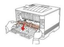
**Step2:** Gently pull the jammed paper out, then c lose the back cover after removing the paper jammed, install a new toner cartridge and then close the front cover; then, the printer will recover printing automatically.
